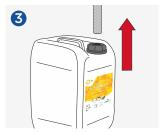
Carefully remove the dishwashing tube out of the RELAVIT Autodish H container.
